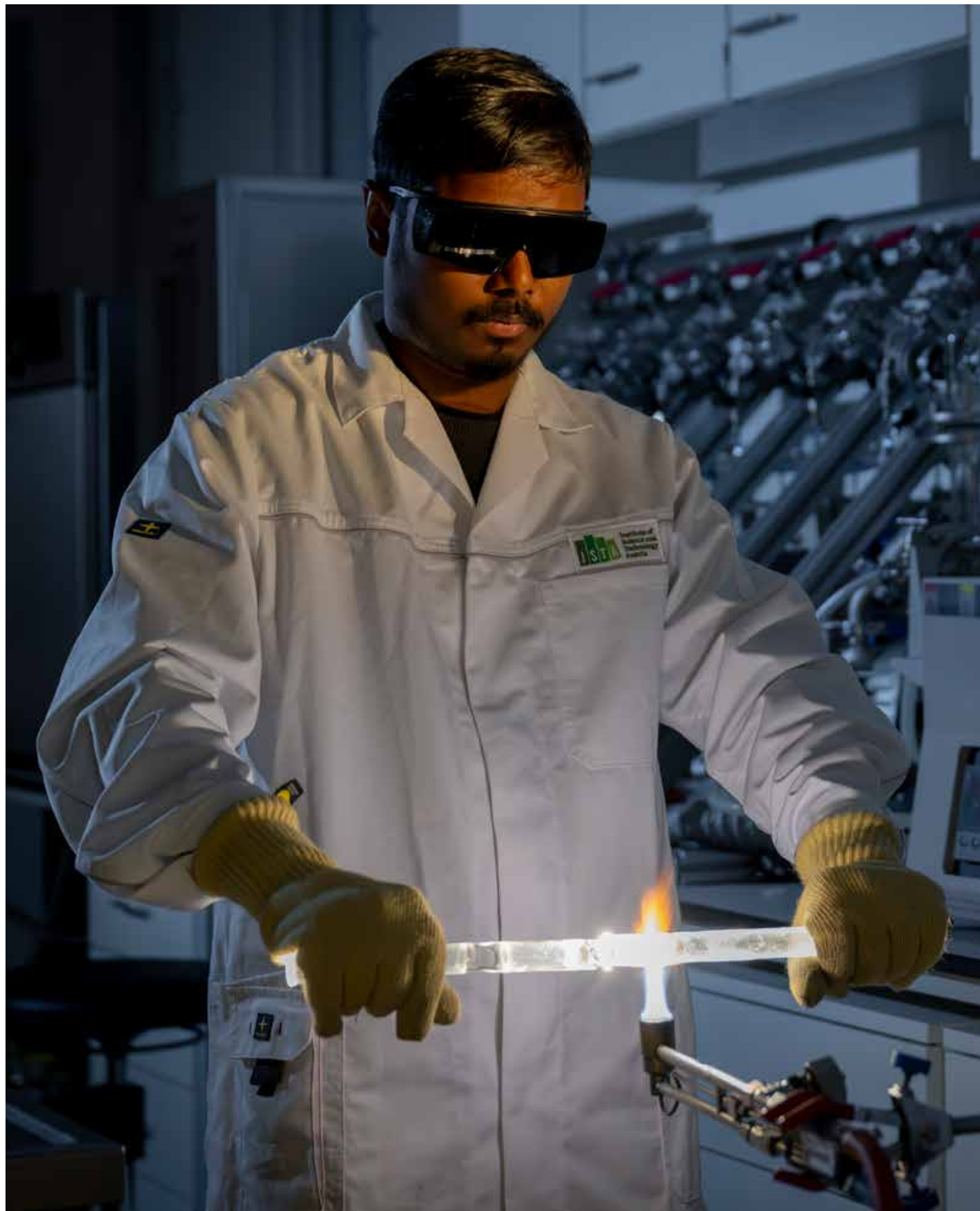
A researcher forms a test tube from molten glass at the WSS Thermolectric Laboratory in Klosterneuburg near Vienna.
