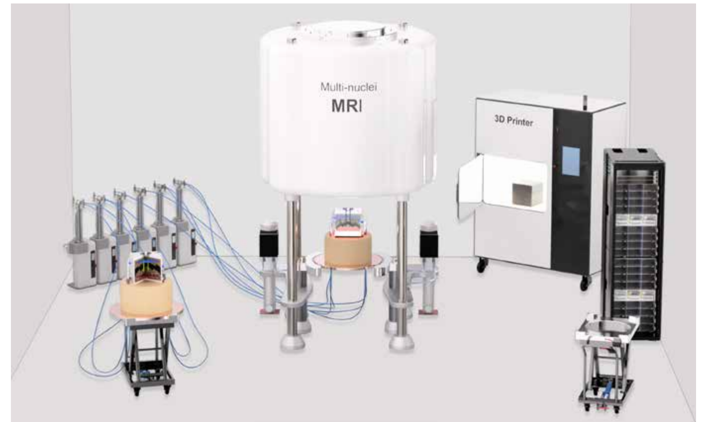
A visualisation of the planned MRI lab: miniature models of geological reservoirs are printed in the 3D printer (right), prepared for the test on an experimental trolley (left) and then placed in the MRI (centre).
