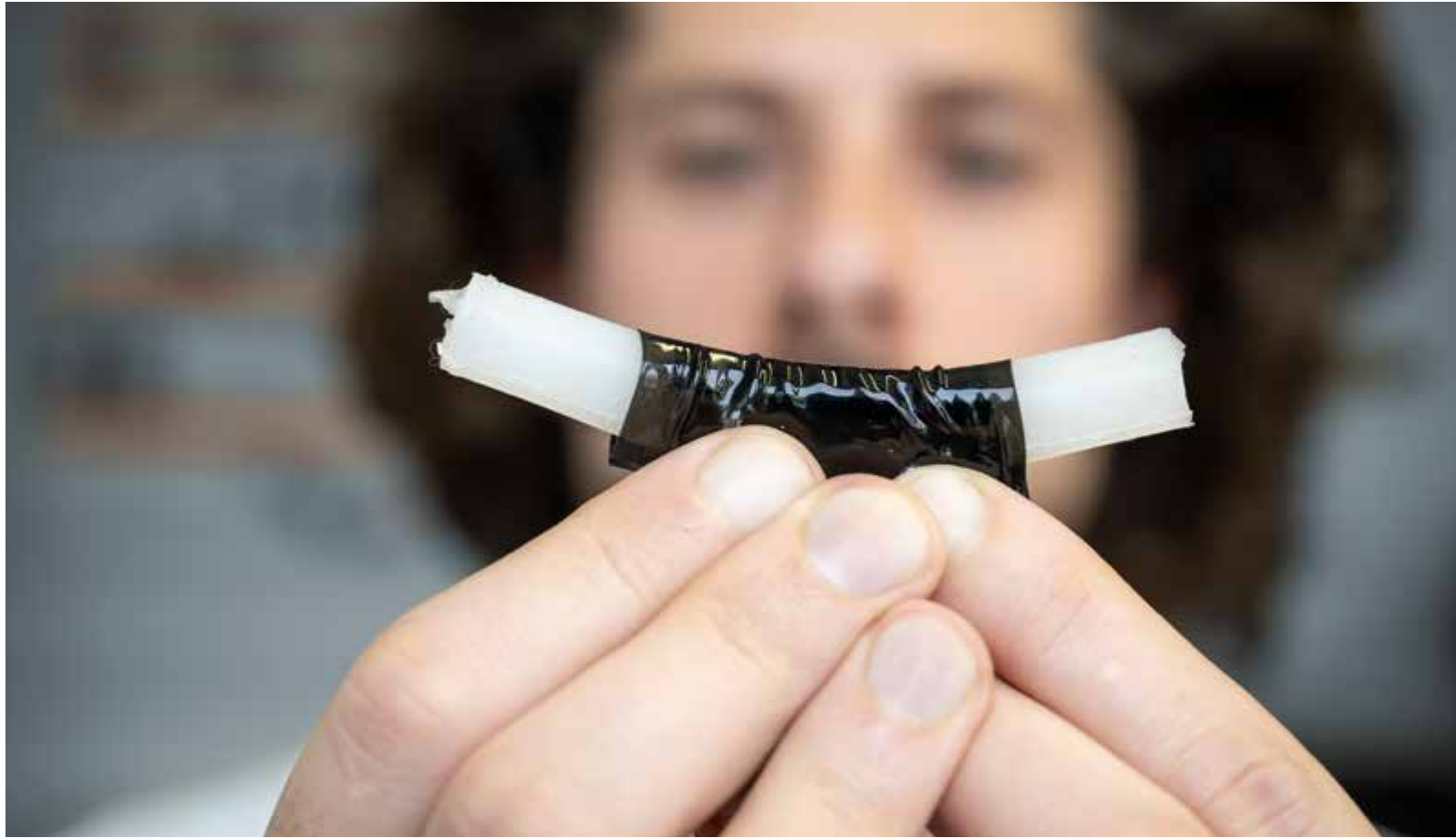
The researchers plan to use the artificial muscle (black) to squeeze and then relax the urethra.
