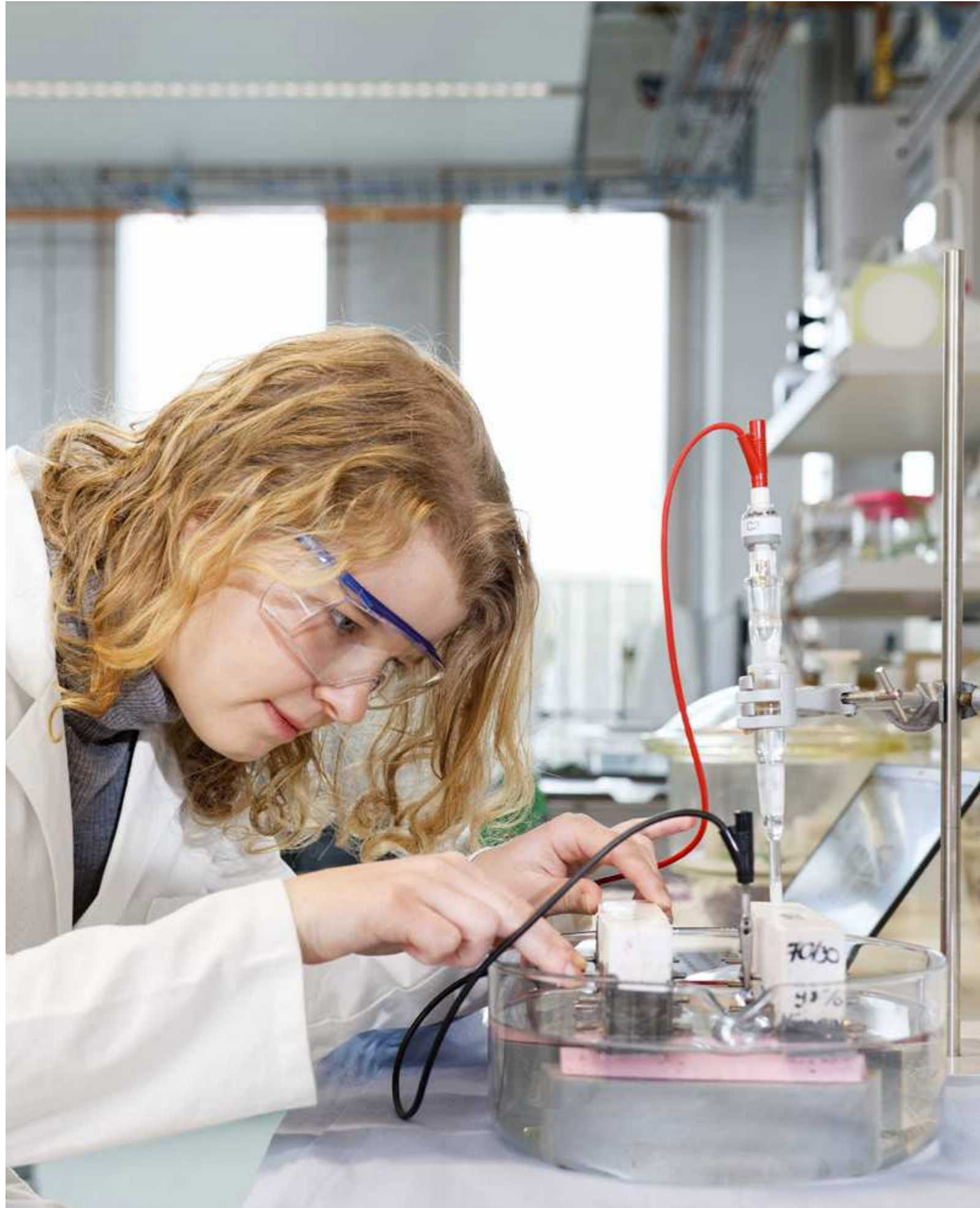
Ueli Angst's research group at ETH Zurich examine small mortar samples to learn more about corrosion processes in reinforced concrete.
