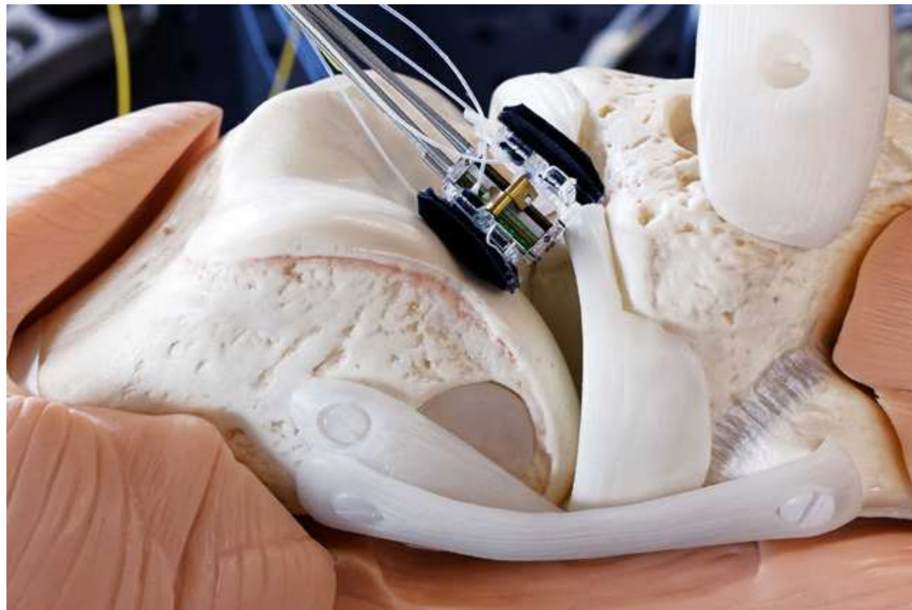
Using a device that resembles an air cushion, the surgical robot can be affixed in the gap of the knee joint, stabilising the laser so that it can cut without moving.
