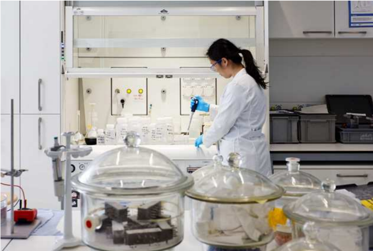
Small mortar samples in glass containers are exposed to various highly specific climatic environments—and then studied under controlled conditions.
