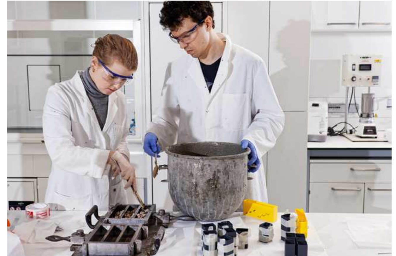
Mixing concrete in the lab: to gain insight into processes occurring inside the material, small concrete blocks are produced and then analysed.
