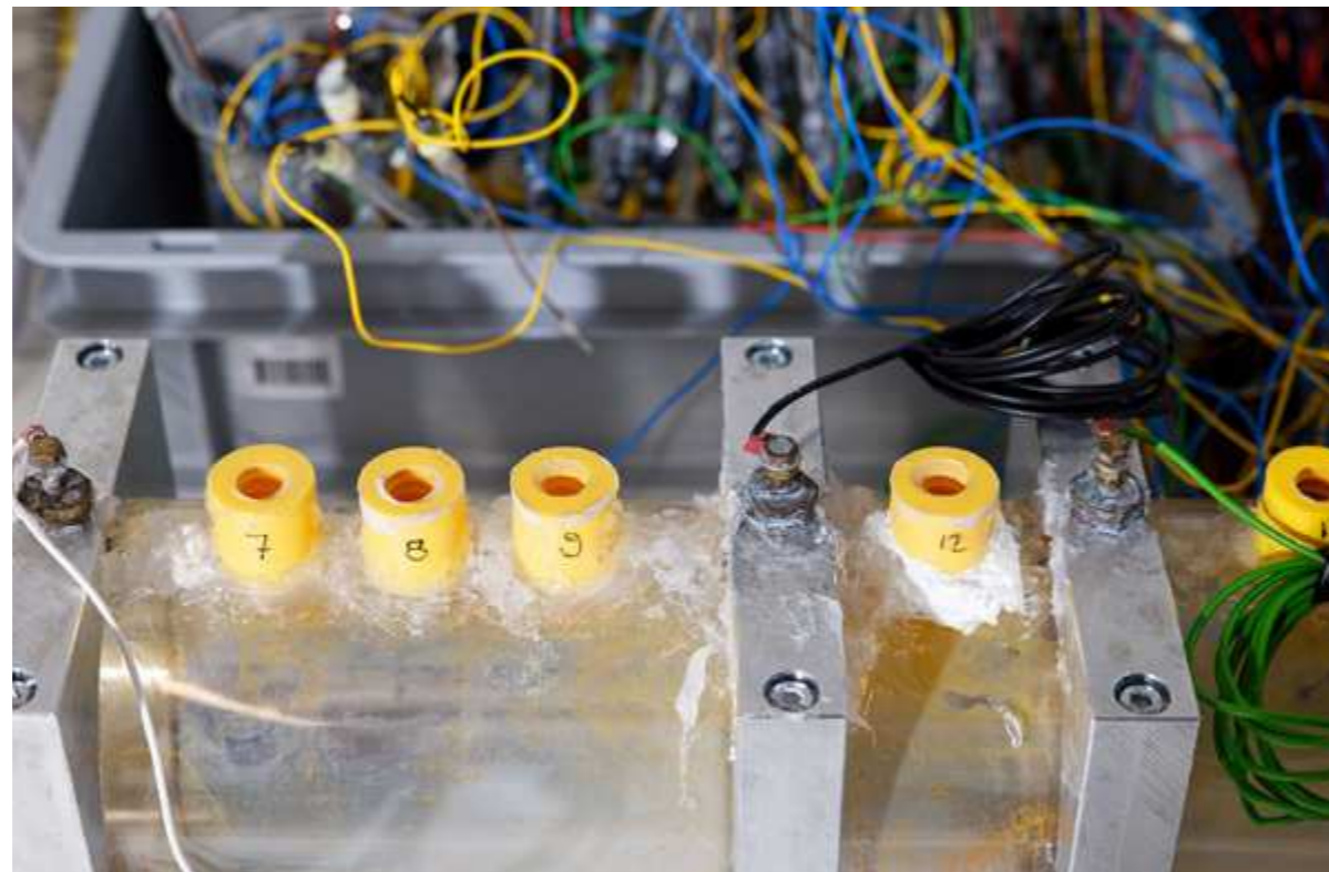
To measure localised corrosion processes on a steel rod, numerous cables are connected to individual measurement electrodes.
