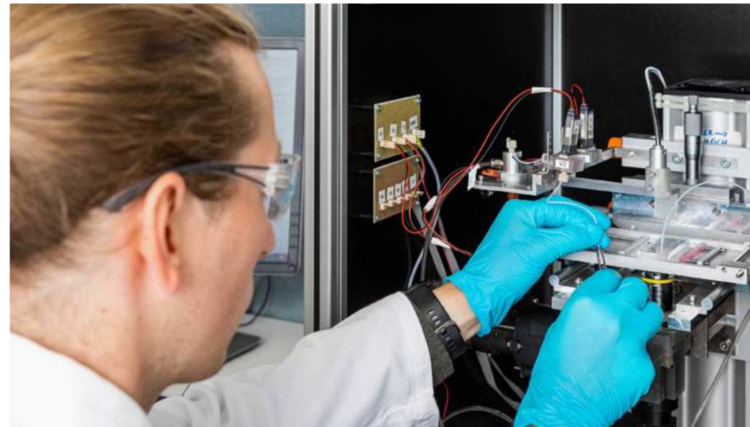
Researchers in Aachen use stop-flow lithography to align maghemite nanoparticles inside the gel rods via a magnetic field during the gel rod production phase itself.
