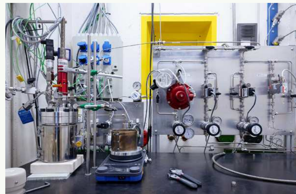
In this test reactor located in a high-pressure chamber, a catalytic reaction is triggered to break down polyethylene admixed with ethylene into the basic building block propylene.
