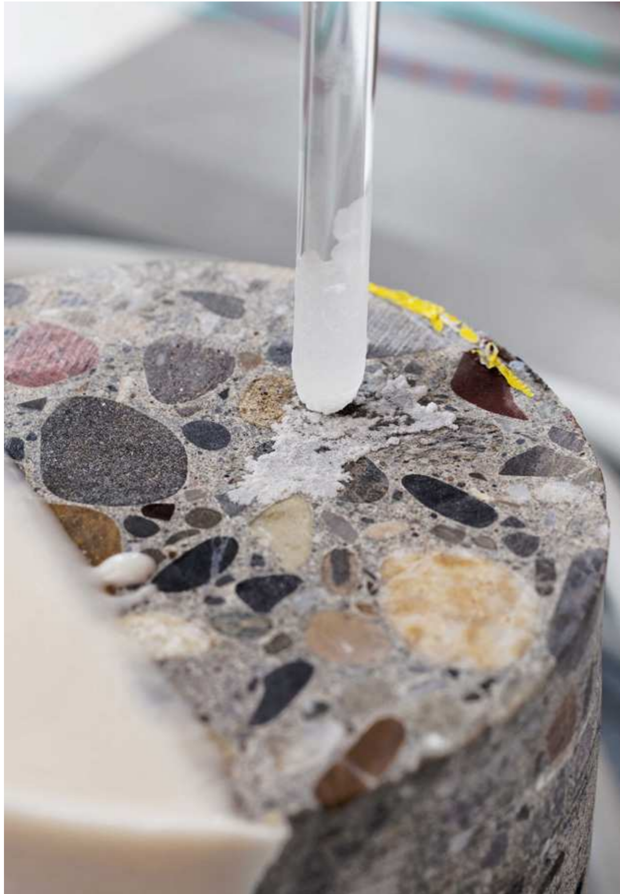
Placing a measurement probe on the surface enables researchers to observe corrosion processes inside the concrete.
