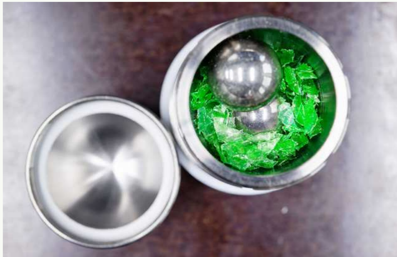
In the cryogenic mill, two balls grind plastic materials to a powder. The temperatures are kept low to prevent the plastic from melting.
